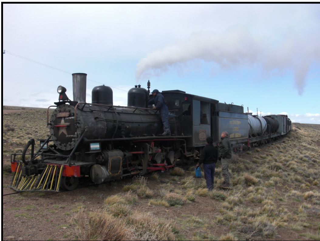
Baldwin No.16 in the middle of the Argentinian Pampa showing the bleak operating environment. Additional water is carried in the tanker wagon behind the tender.
