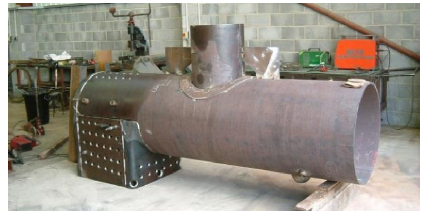
Photo taken at Bennetts Boiler works showing the partially completed boiler for No.778. The new boiler for 762 will be of similar welded construction with flanged throat and backhead.
