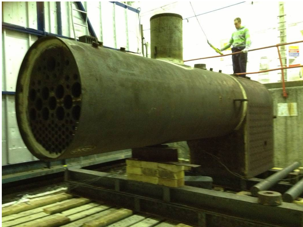
Lyn's Boiler being located into JJ Castings oven – Photo courtesy of JJ Castings Ltd
