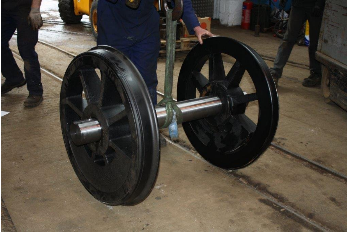
Above: The completed operations showing the driving wheels attached to their axles.
