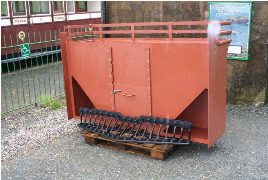
Left: The completed bunker and a cowcatcher sits at Woody Bay ready for the Vintage Weekend.
